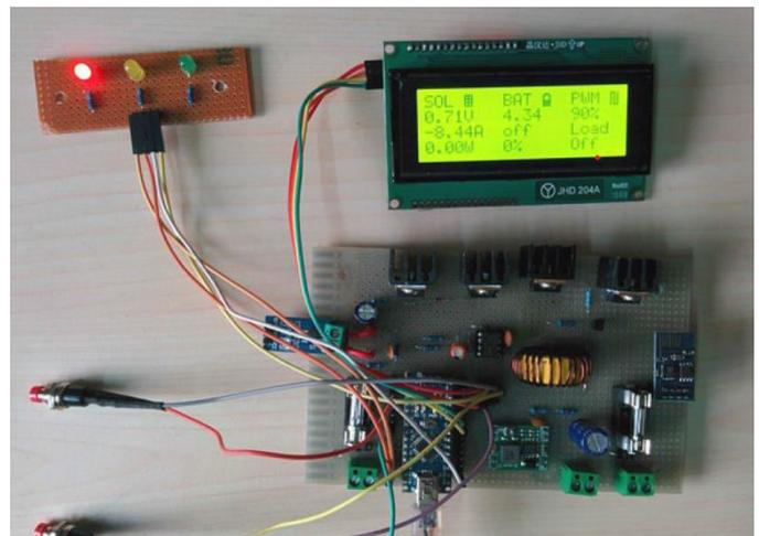
Fig 03. The above fig shows the complete charging system its also provided with reset button in case of program structed we can use of it.
