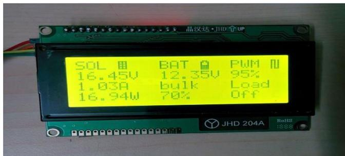
**Fig.01 LCD Display With battery parameters indication**
