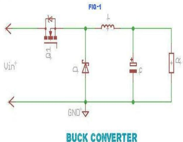
In our case, the input source is a 50W solar panel and load is a 12V lead-acid battery. From the earlier discussion, we have concluded that a buck converter consists of 1.Inductor 2.Capacitor 3.MOSFETS
