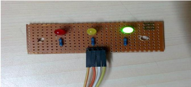
Above fig shows that this project also contains the LED charging level indications of the battery, With the help of led's we can see the battery charging level indication.
