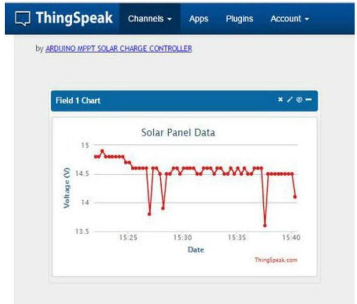
The above fig shows the data chart uploaded to the thingspeak.com voltage vs time. With the help of this we can track the solar voltage remotely from anywhere.
